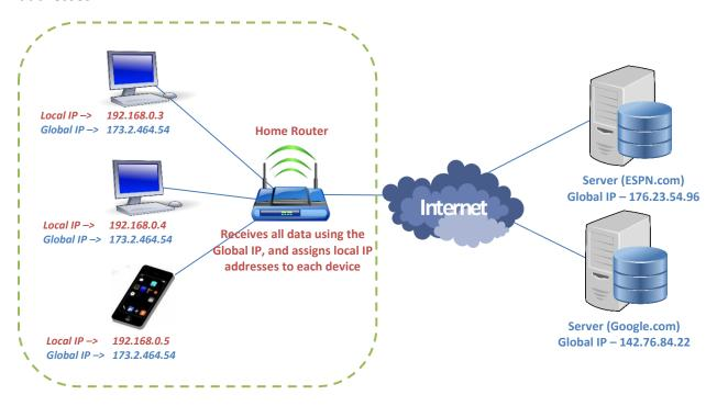
Each device can have two separate IP addresses, a local and a global. A local IP is assigned from your local network router (i.e. – the box in the closet). The global IP is assigned by your Internet Service Provider (ISP) (i.e. – Verizon, comcast, cable, etc.).
