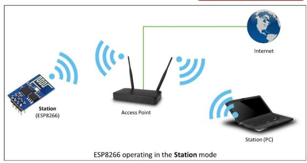
An access point is usually integrated with a router to provide access to the internet. The access point is recognized by a SSID (Service Set Identifier), that essentially is the name of network you select when connecting a device (station) to the Wi-Fi.
