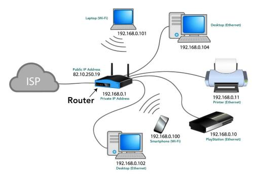
Being there are only a limited number of global IP addresses (there are more devices in the world than addresses), each network only gets one **global IP**. Since your network can have multiple devices within it, like laptops and phones, the router's job is to assign each device a **local IP** address, one that the outside world cannot see. The router uses these local addresses to distribute the data to the correct device within the network.
